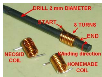
SMD 56nH coil used for L8-L11
